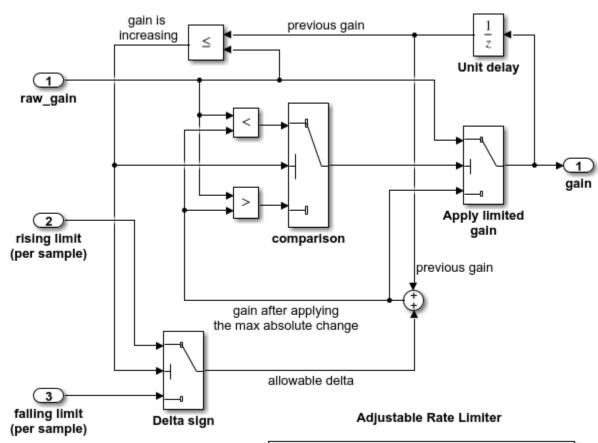
This component implements a rate limiter where the maximum and minimum slew rates are input signals
